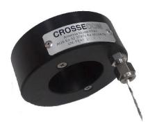
The antenna, mounted conveniently on the dispensing nozzle spout, comprises a small loop antenna with its low power electronic components. It is connected to the reader (mounted inside the pump housing) via a special petroleum resistant cable.
