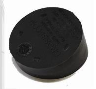
This is a small batteryless electronic data storage unit (20-50mm in diameter) epoxied to the vehicle near the fill pipe. It can contain information such as vehicle details, owner identification, driver identification, fuel type etc.
